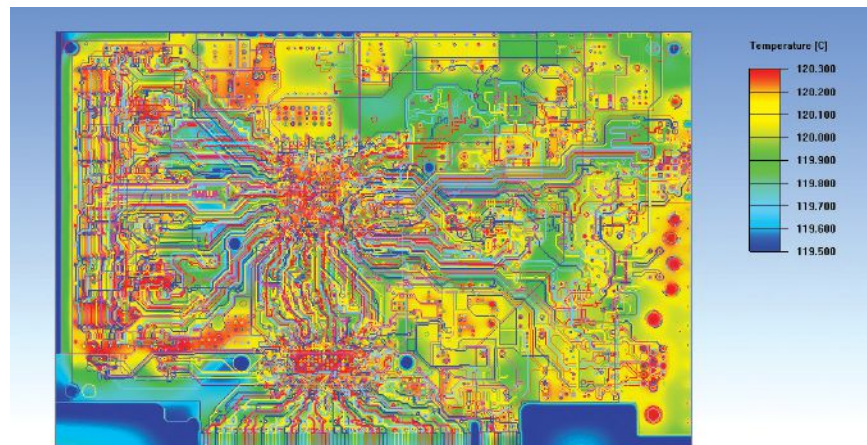
ANSYS Icepak lets you perform transient and steady-state thermal behaviors. Shown here is the heat map of a PCB generated in Icepak. Image courtesy of ANSYS.
